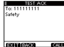
④ While transmitting the acknowledgement call, the screen shown below is displayed, and then returns to the normal operating mode.
