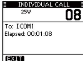
Or, when the acknowledgement 'Unable to comply' is received, alarm sounds and the screen below is displayed.
