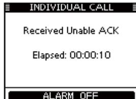
Push [ALARM OFF] to stop the alarm. Then push [EXIT] to return to the operating channel (before you entered the MENU screen).
