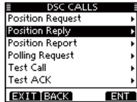
② Select a desired Position Request call to reply to, using dial or [▲]/[▼], then push [ENT].
