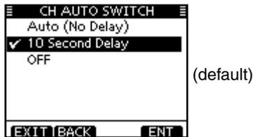
**Auto (No Delay):** After receiving a Distress call, and [ACPT] is pushed on the confirmation screen, the transceiver immediately switches to Channel 16.
