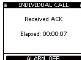
Push [ALARM OFF] to stop the alarm and then select the intership channel specified in step ③.
