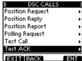
② Select a desired Test call to reply to, using dial or [▲]/[▼], then push [ENT].
