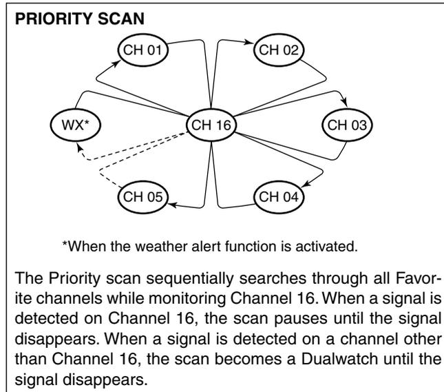
Set the Favorite channels (scanned channel) before scanning. Clear the Favorite channels which inconveniently stop scanning, such as those for digital communication use. (Refer to the next page for details.)
