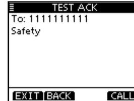
When “TEST ACK” is set to “Auto,” the transceiver automatically replies to the Call. In that case, both the TX and RX calls are stored in the Transmitted and Received Call Logs.
