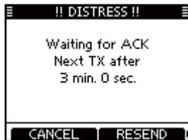
⑥ After receiving an acknowledgment call, push [ALARM OFF] then reply using the microphone.
