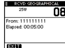
When no GPS receiver is connected or if there is a problem with the connected receiver, all Geographical Area Calls are received, regardless of your position.
