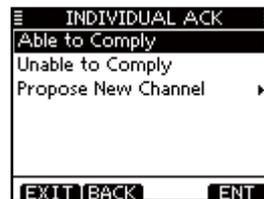
When “INDIVIDUAL ACK” is set to “Auto (Unable),” the transceiver automatically replies to the Call. In that case, both the TX and RX calls are stored in the Transmitted and Received Call Logs.
