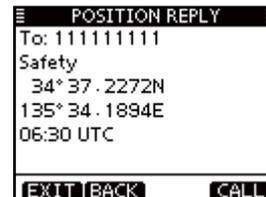
④ While transmitting the reply call, the screen shown below is displayed, and then returns to the normal operating mode.
