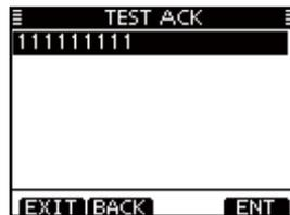
③ The Test ACK confirmation screen is displayed. Push [CALL] to transmit the acknowledgement call.
