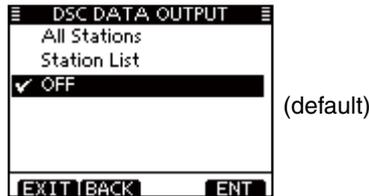
All Stations: Outputs the call from any vessel from the NMEA Output port.
